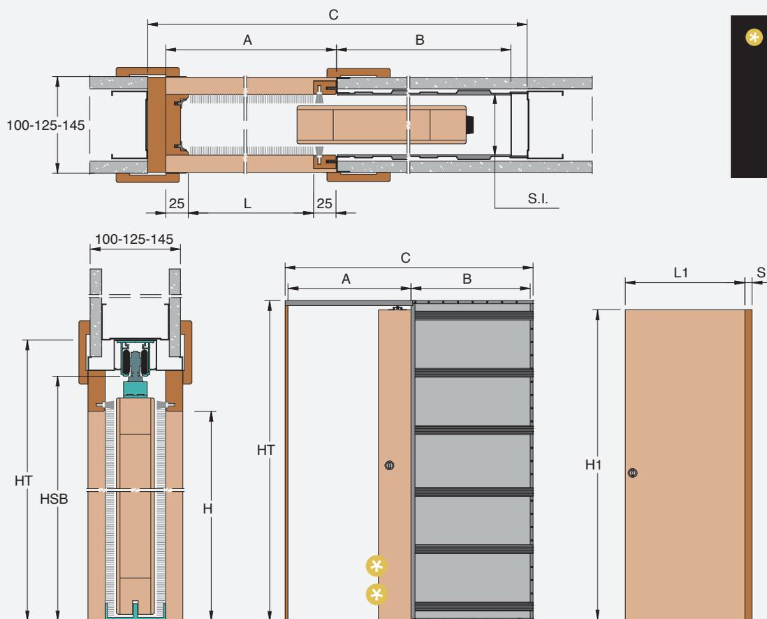
**\*\* The panel fully enters the wall cavity.**
