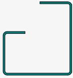
The aluminium horizontal passage profile can be painted. It has three holes to be fixed with screws and allows motor's inspection.
